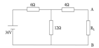
Calculate the maximum power, that can be transferred from the source in the given circuit.
