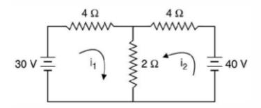
Determine the current  $i_2$  of the given network using loop analysis.
