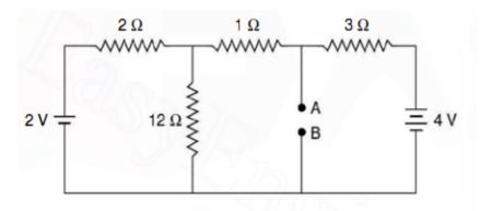
Calculate the Thevenin equivalent resistance between A and B in the given circuit.
