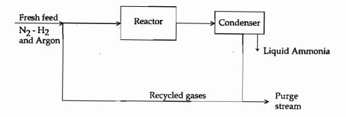
All of the ammonia formed is separated by condensation and the unconverted gases are recycled to the reactor. The fresh feed of  $N_2-H_2$  mixture contains 0.17 mol Argon per 100 mol  $N_2-H_2$  mixture. The concentration of Argon in the gases entering the reactor is to be kept below 6 mol Argon per 100 mol  $N_2-H_2$  mixture. Estimate the minimum fraction of the recycle that must be purged.
